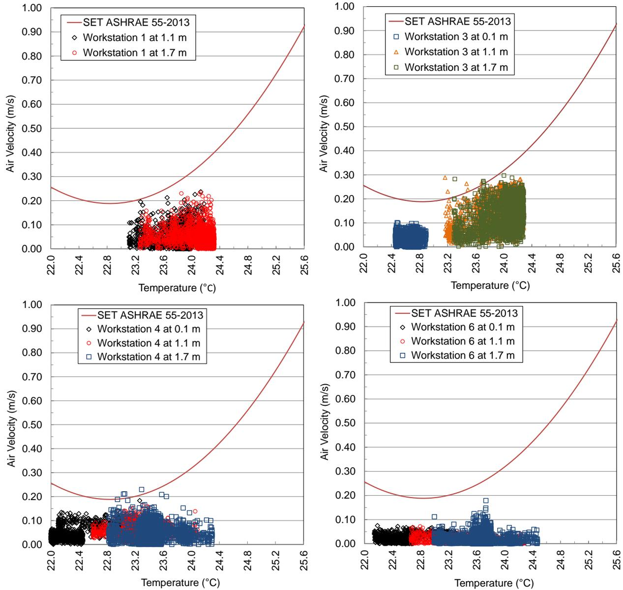
Figure 45: Limit to air speed for Case 5, Test 21
