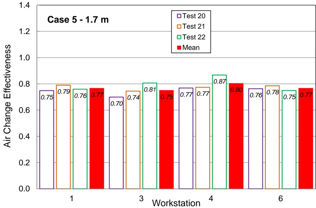
Figure 34: Measured values ACE for case 5 at standing breathing height of 1.7 m.
