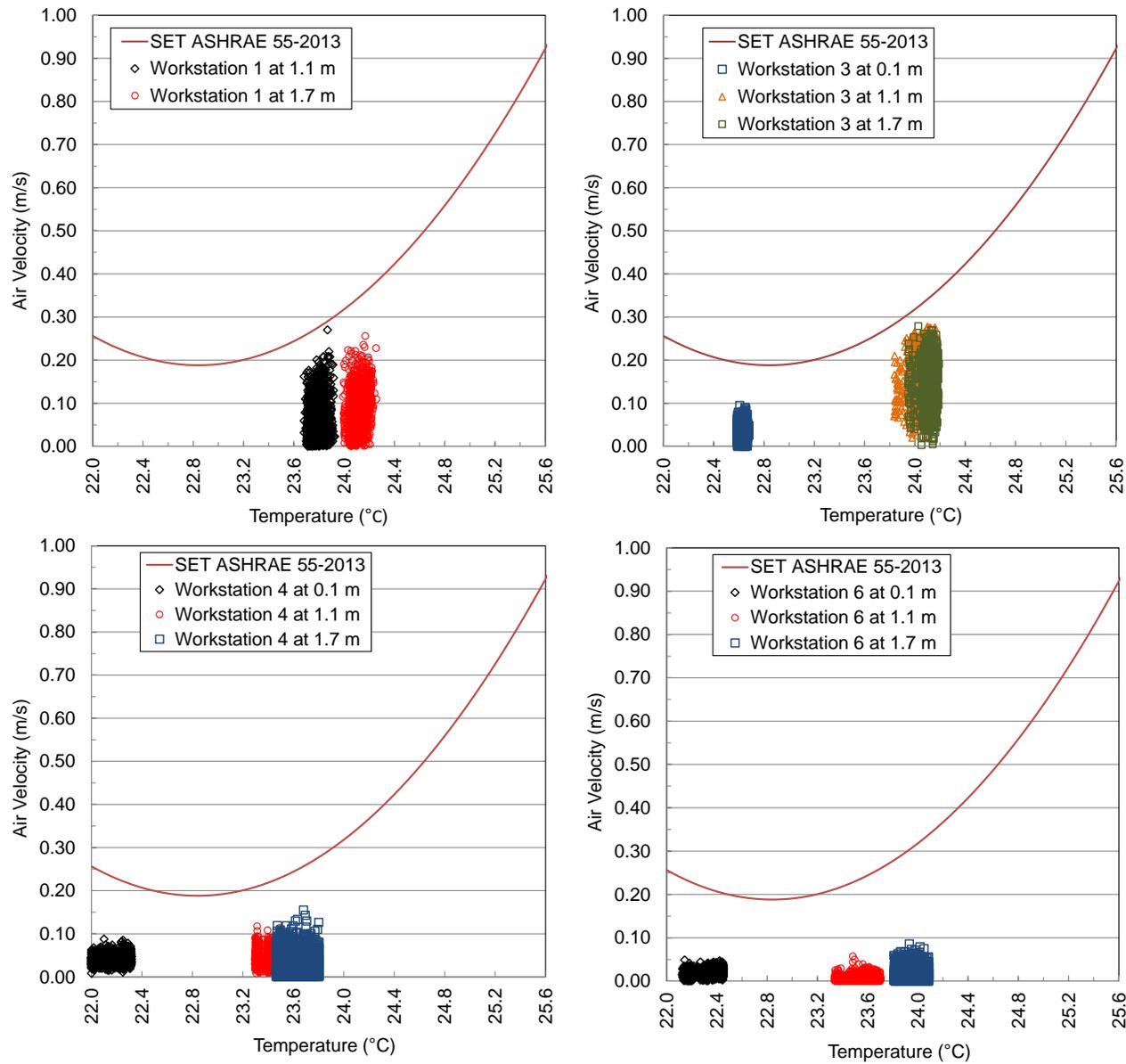
Figure 43: Limit to air speed for Case 3, Test 11
