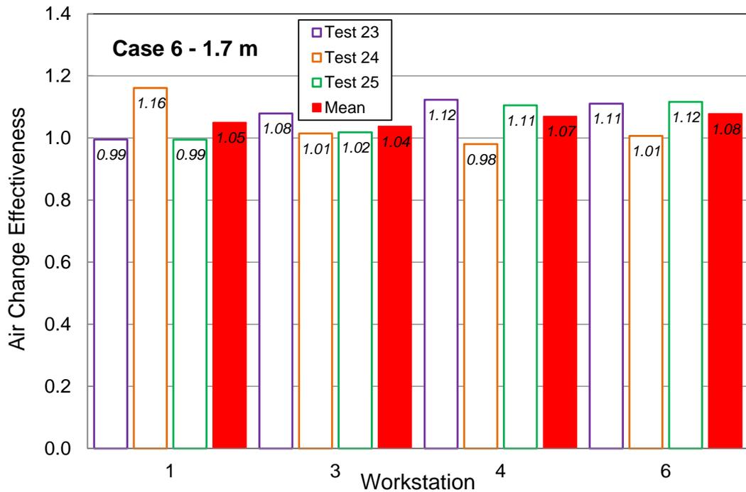
Figure 36: Measured values ACE for case 6 at standing breathing height of 1.7 m.
