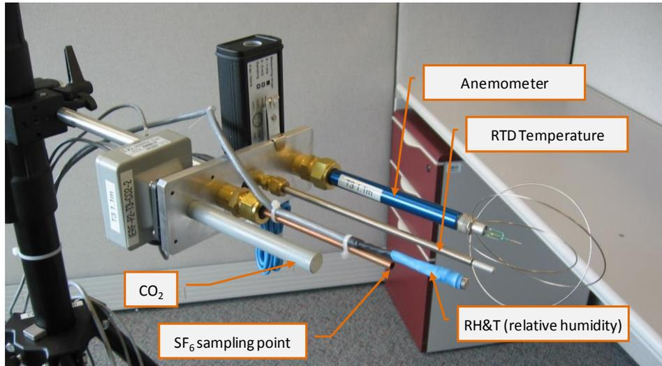
Figure 14: Sensor holder with sensors attached. A PVC pipe was attached to the back end of the copper pipe for SF<sub>6</sub> sampling.
