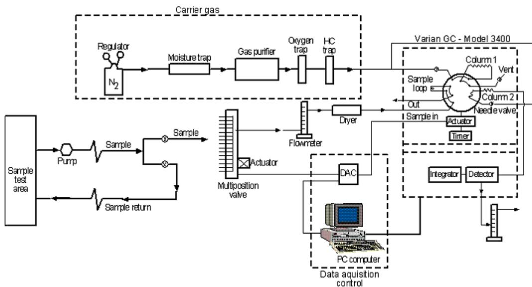
Figure 4: Schematic diagram of a multi-position tracer gas sampling system.
