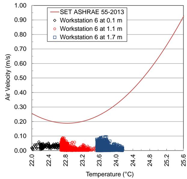
Figure 41: Limit to air speed for Case 1, Test 2
