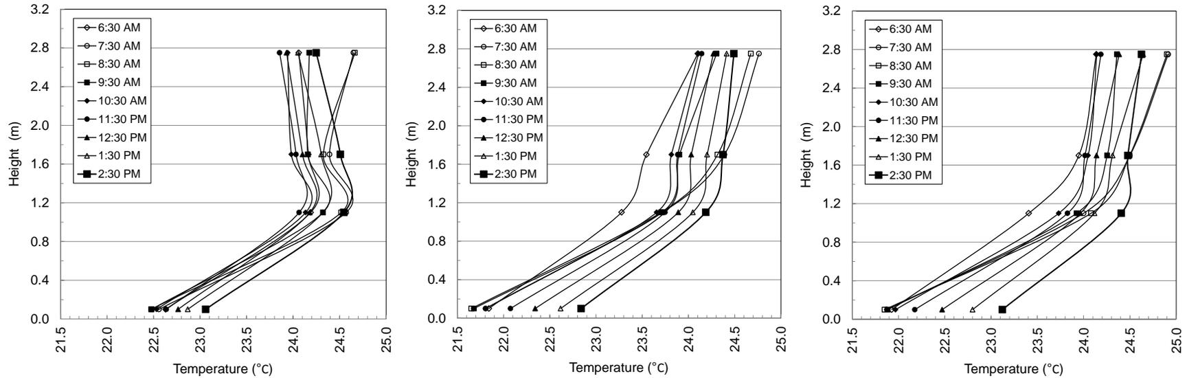
Figure 39: Examples of vertical temperature profiles in workstations 3 (left), 4 (centre), 6 (right) for Case 5
