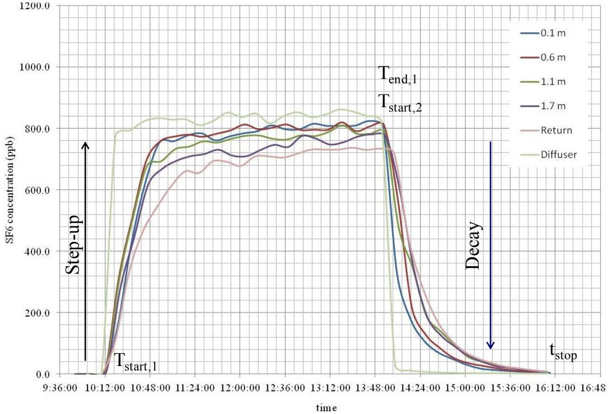
Figure 15: Tracer gas concentration variation - step-up and decay
