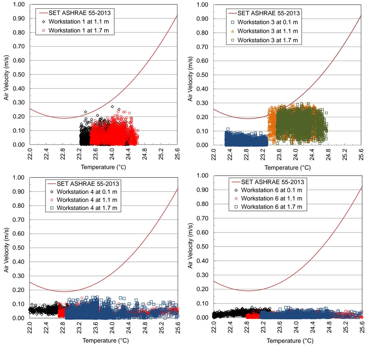
Figure 44: Limit to air speed for Case 4, Test 17
