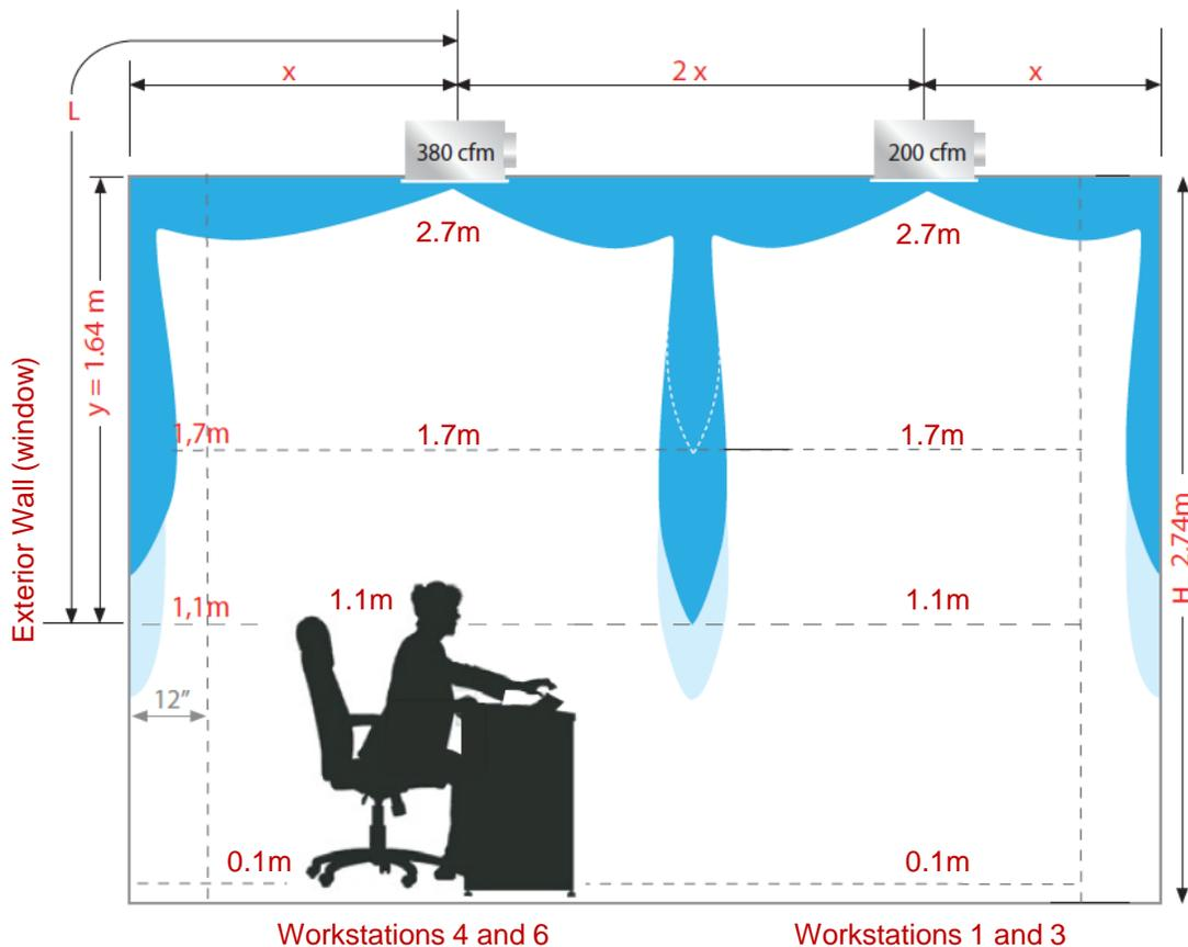
Figure 13: Measurement heights in the vicinity of exterior wall (window), exterior workstation 4 & 6 and interior workstations 1 & 3
