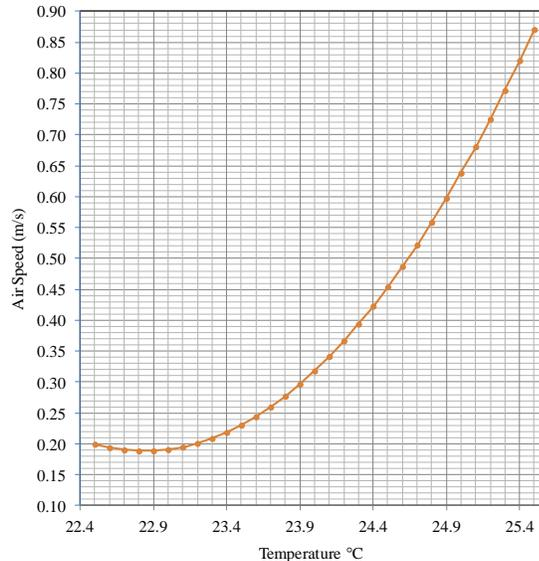
Figure 40: Equal-SET curve for 0.6 clo and 1.1 met (ASHRAE 55-2010).
