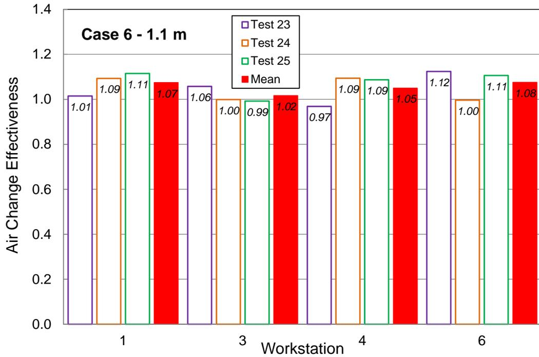
Figure 35: Measured values ACE for case 6 at seated breathing height of 1.1 m.
