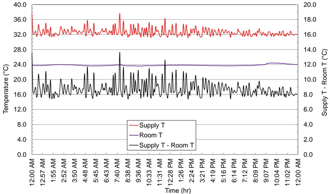
Figure 20: Supply and space temperature distribution – 29/03/2016
